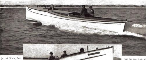
Jr., of New Bedford, Mass. She is 29 feet in length. with a beam of 7 feet 2 inches and an extreme draft of 26 inches. The motor installed is a 6-cylinder, 60 h.p. Loew-Victor with full automobile control, including electric self-starter, electric
