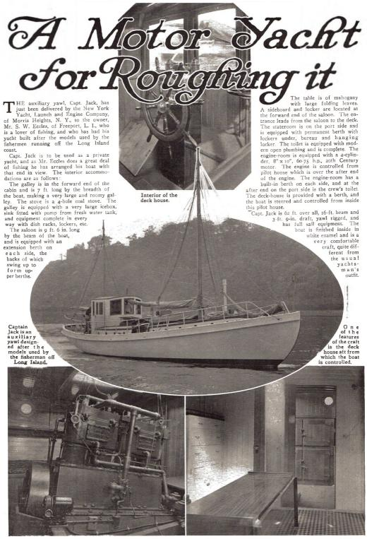
Captain Jack is powered with a 4-cylinder 8" x 10" Twentieth Century motor developing 60 to 75 h.p.
