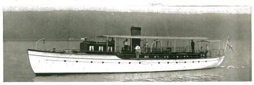
Drusilla is 83 feet long with a beam of 14 feet and a 4-foot draft.
